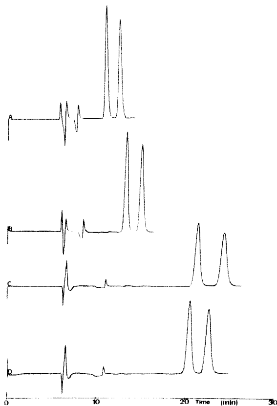
Fig. 3. Chromatograms of N-0437 (390 \mu\text{g/ml} ) obtained under various conditions: (A) eluent, hexane-ethanol (85:15), temperature 0°C, flow-rate 0.5 ml/min, PO point 26; (B) eluent, hexane-ethanol (90:10), temperature 0°C, flow-rate 0.5 ml/min, PO point 28; (C) eluent, hexane-ethanol (95:5), temperature 0°C, flow-rate 0.5 ml/min, PO point 31; (D) eluent, hexane-ethanol (95:5), temperature 10°C, flow-rate 0.5 ml/min.
